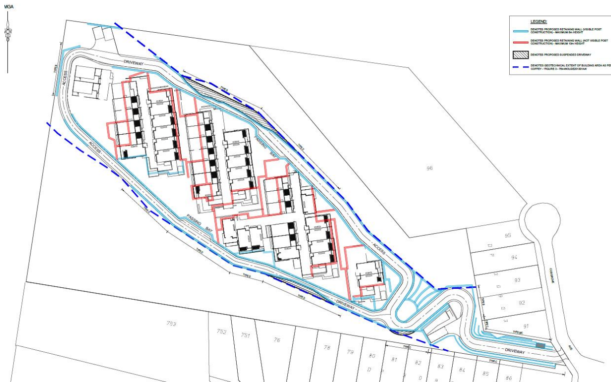
Figure 27: Retaining Wall Layout Plan extract
